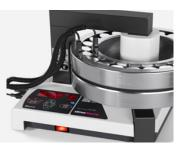
The best way to avoid unwanted stresses when assembling interference-fit parts is to heat the outer part just enough to produce a temporary clearance. simatherm induction heaters allow this to be done precisely, evenly, quickly and efficiently. Other methods of heating are slower, less controlled and can cause more harm than good to bearings.
