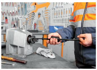
Knowhow: using a Seal Puller SP 50 to remove a radial seal from a gearbox without damaging the housing or shaft.
