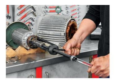
The Twin Puller TP 150 does it: a tightly seated bearing of an electric motor is removed without risking damage to the housing or the shaft.
