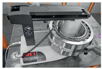
The roller bearing placed around the coil of an IH 210 heater is heated by induction. A simatool Bearing Handling Tool is in place to position the bearing on the shaft, once the specified mounting temperature is reached.
