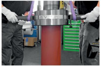
The Bearing Handling Tool BHT allows the heavy, pre-heated roller bearing to be safely lifted and accurately positioned on a turbine shaft.
