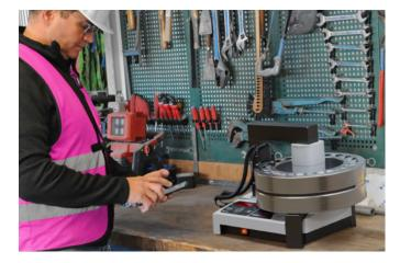
The simatherm IH 045 is operated via the APP simatec WoM. The spherical roller bearing is heated with the two-sensor mode, to avoid mechanical stresses in the bearing.
