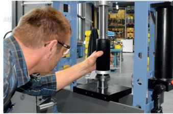
The FT-P is the ideal solution for installations with greater forces, as the tool can be used on a press. High-quality aluminum rings that do not deform even with press-in forces of 5 tons.
