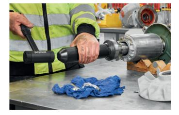
The Fitting Tool FT 33 ensures that the mounting force is evenly distributed across the inner and outer rings of the bearing and therefore does not stress the rolling elements.
