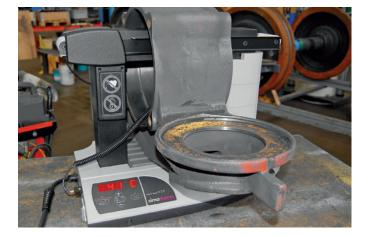
Working on a train wheel-set, the high-performance induction heater IH 210 heats a massive bearing housing to allow a bearing to be inserted.
