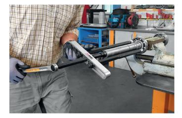
With the aid of extensions, the BP 160 dismounting tool kit also makes it possible to dismount hard-to-reach bearings easily and professionally.
