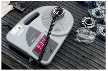
The portable VOLCANO IH 025 is used for the installation of gear shafts. For this purpose, a tapered roller bearing is heated to the desired temperature using the temperate monitoring system.
