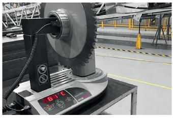
The induction heater IH 070 is the ideal choice for heating the return sprocket of the step chain of an escalator.
